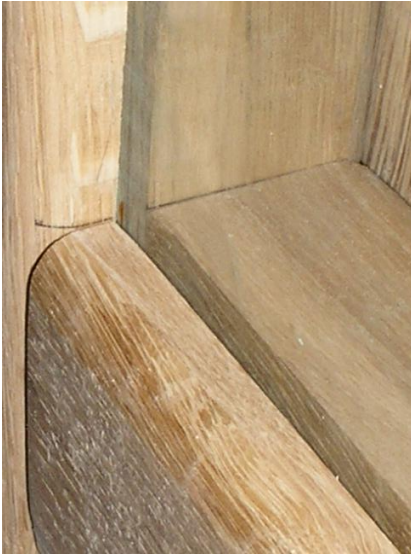
Slots routed for glass and edges rounded prior to varnishing
