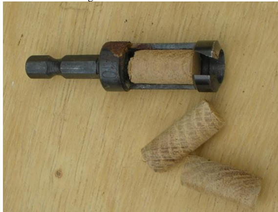
Coring tool and cores to hide screw head
